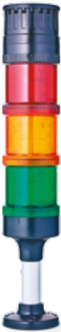
Order number: ECO70-Q31 Colours: red/orange/green Function: LED steady beacon, buzzer steady or pulsing tone Nominal voltage: 24 V AC/DC Type of mounting: Tube mounting (100 mm tube length)
