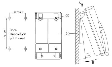
Place the telephone in the upper latches (A), swing it downwards until the lower latches audibly engage(B).
