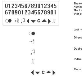
The two uppermost lines display numbers or the menu settings. The lower line displays pictograms that correspond to the functions.
