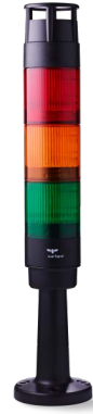
Order no.: CT5-Q31 Colours: red/amber/green Function: LED steady beacon, Piezo buzzer module, one of eight tones can be selected with a dip switch Nominal voltage: 24 V DC Type of mounting: Tube mounting (100 mm tube length)
